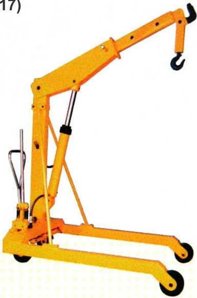
Manually Mobile Floor Crane Capacity-500 Kg To 2000 Kg Min Hook Height -300 Mm Max Hook Height -3000 Mm
